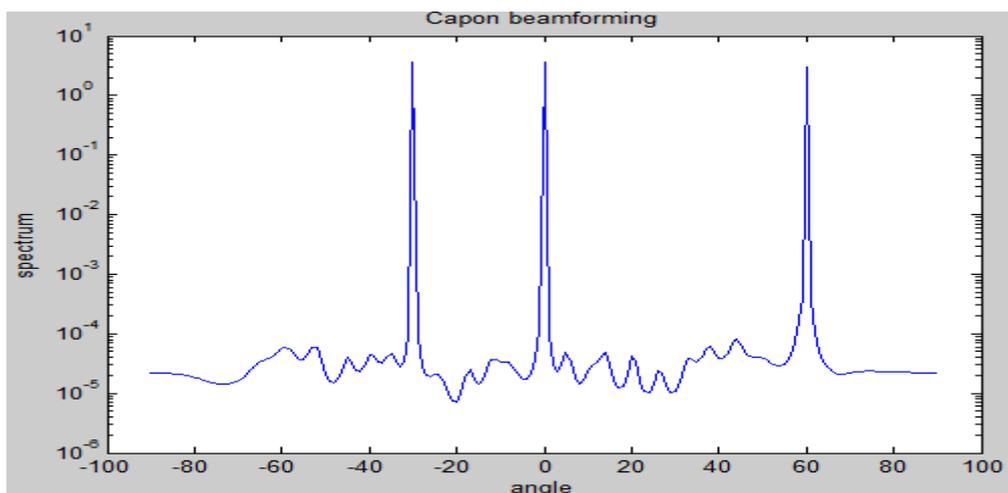
Figure 4.1.1  $I = 3, M = 32, SNR = 20, \phi_1 = -30^\circ, \phi_2 = 0^\circ, \phi_3 = 60^\circ$
