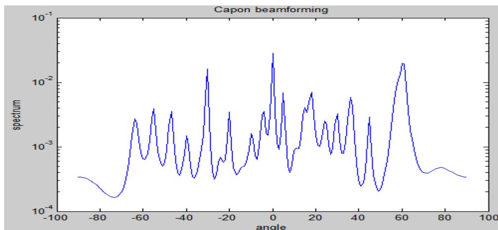
Figure 4.1.2  $I = 3, M = 32, SNR = 0, \phi_1 = -30^\circ, \phi_2 = 0^\circ, \phi_3 = 60^\circ$
