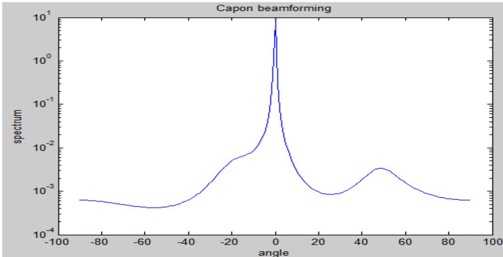
Figure 4.1.3  $I = 3, M = 4, SNR = 20, \phi_1 = -30^\circ, \phi_2 = 0^\circ, \phi_3 = 60^\circ$
