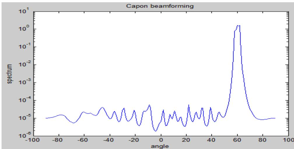
Figure 4.1.4  $I = 3, M = 32, SNR = 20, \phi_1 = 58^\circ, \phi_2 = 60^\circ, \phi_3 = 62^\circ$
