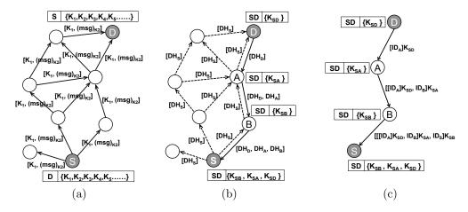
Figure 2: Protocol Overview. (a) Source discovers destination using keys from keyed hash chain; (b) Additional use of broadcast message for Diffie-Hellman key exchange. Unicast is used to forward Diffie-Hellman public keys of en-route nodes back to the source; (c) Verifying the individual connectivity of the path using encrypted topology information
