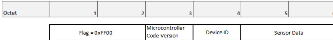
Figure 15: Message structure between sensorboard and laptop
