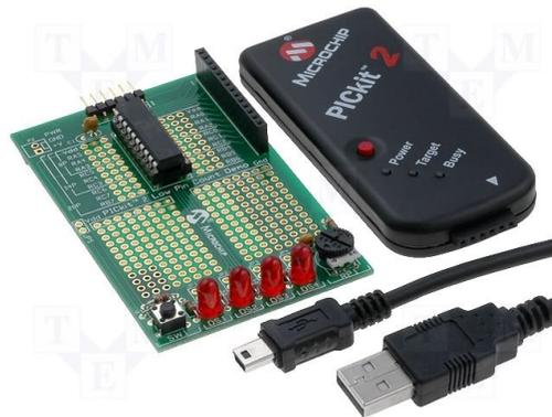
Figure 12: PICKit 2 demoboard and programmer
