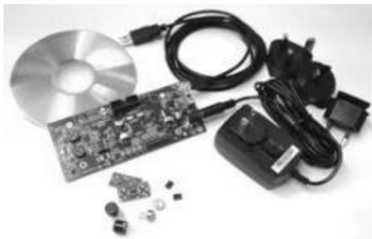
Figure 29 E2v metal oxide semiconductor gas sensor evaluation kit
