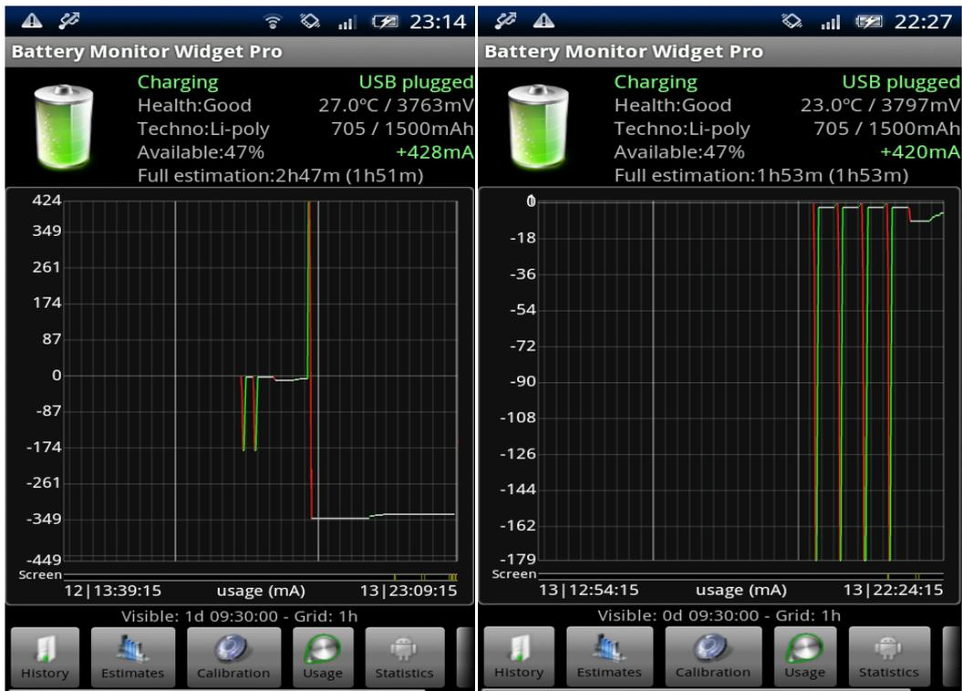
**Figure 22 Power consumption without and with auto method**
