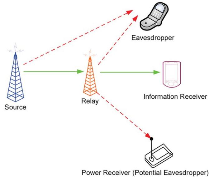
Figure 3.1. a SWIPT system model in relaying networks [41]
