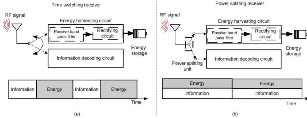
Fig2.6 Typical receivers for SWIPT
