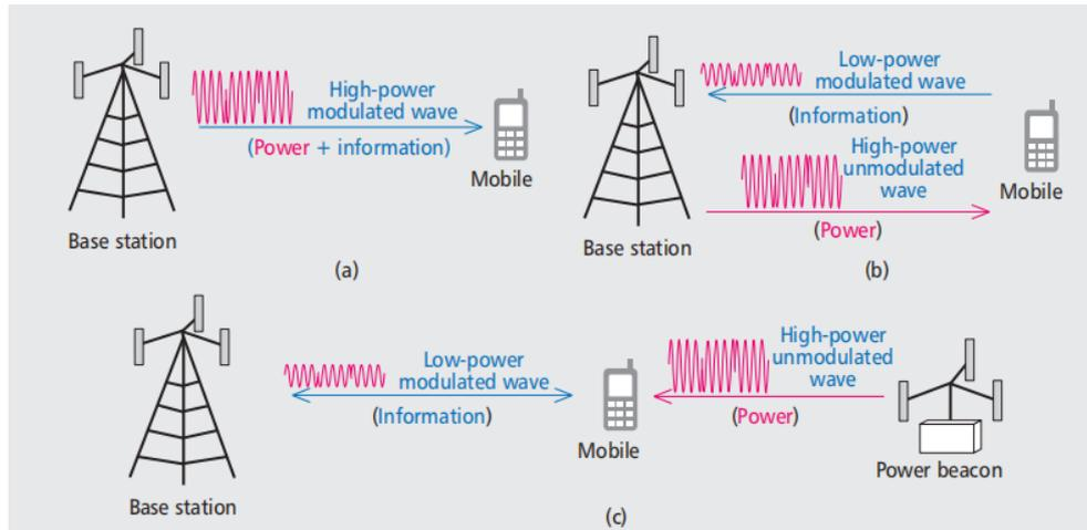
Fig2.5 Typical model of SWIPT technology [10]
