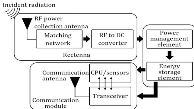
Fig2.4 Block diagram of RF-EH technology receiver [8]
