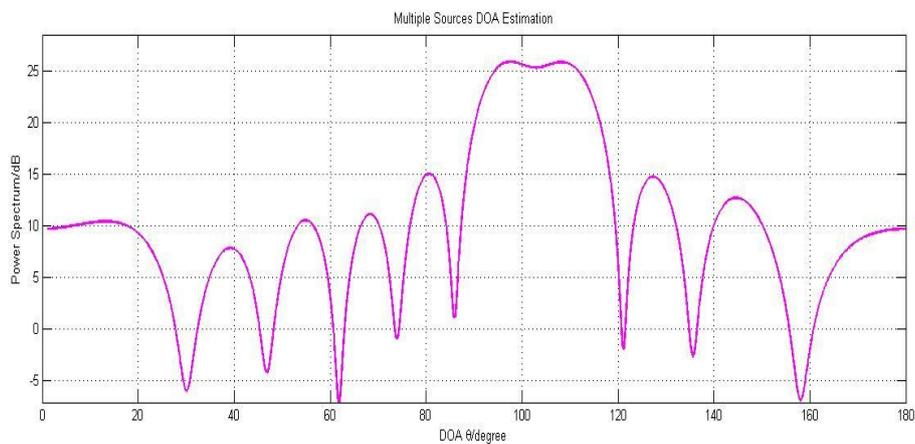
**Figure 4.2.4** Two sources conventional FFT method with close direction angle
