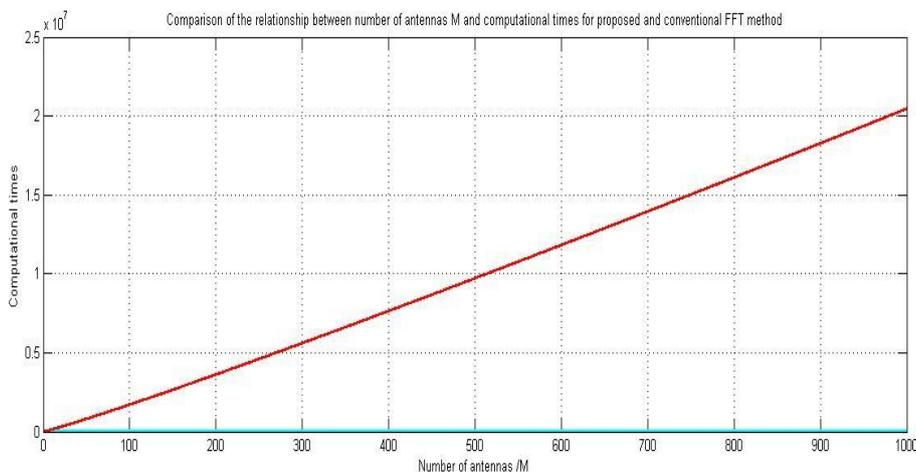
**Figure 4.4.4** Antenna number  $M$  vs. Computational times when  $z = 1024$
