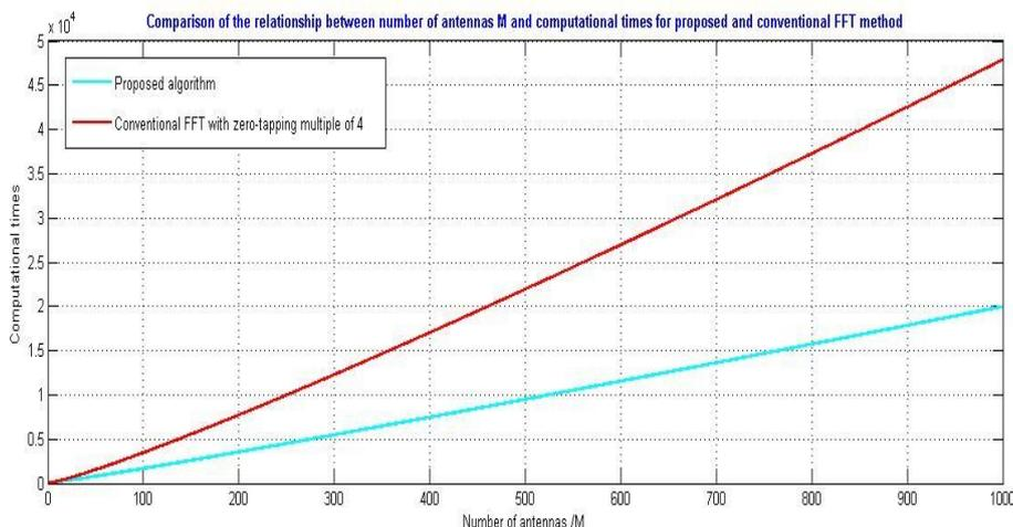
**Figure 4.4.3** Antenna number  $M$  vs. Computational times when  $z = 4$
