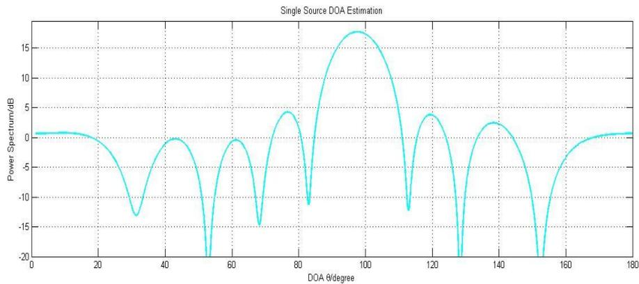
**Figure 4.2.2** Single source conventional FFT method with  $z=1024$
