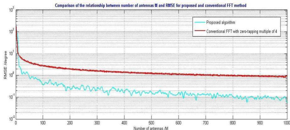
**Figure 4.4.2** Antenna number  $M$  vs.  $RMSE$  for proposed algorithm and conventional FFT
