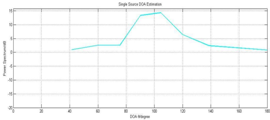
**Figure 4.2.1** Single source conventional FFT method with  $z=1$
