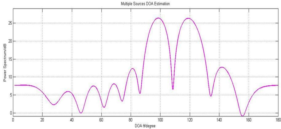
**Figure 4.2.3** Two sources conventional FFT method with sufficiently far direction angle
