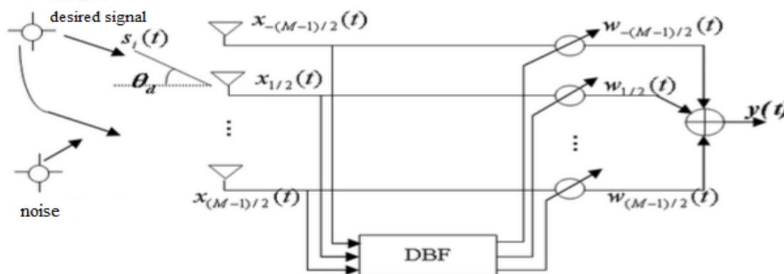
Figure2.1.1 Beamforming technic
