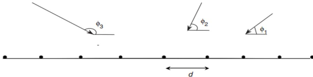
Figure 2.2.1 ULA antenna model and steering vector with different direction
