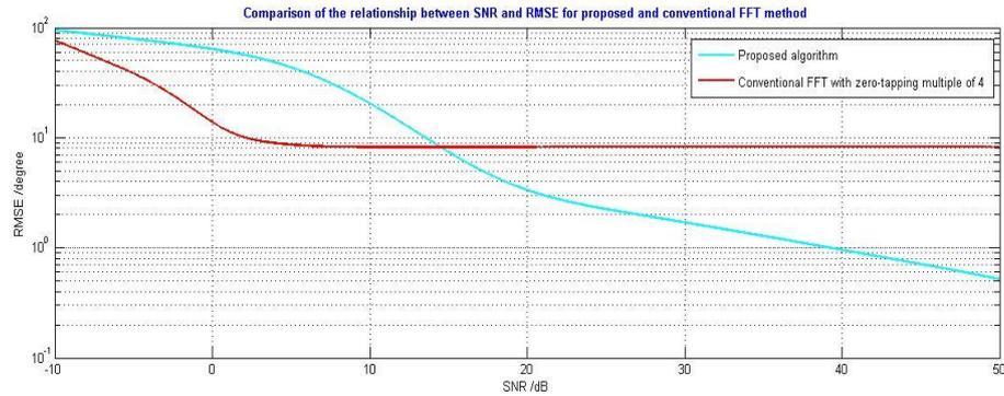
**Figure 4.4.1**  $SNR$  vs.  $RMSE$  for proposed algorithm and conventional FFT
