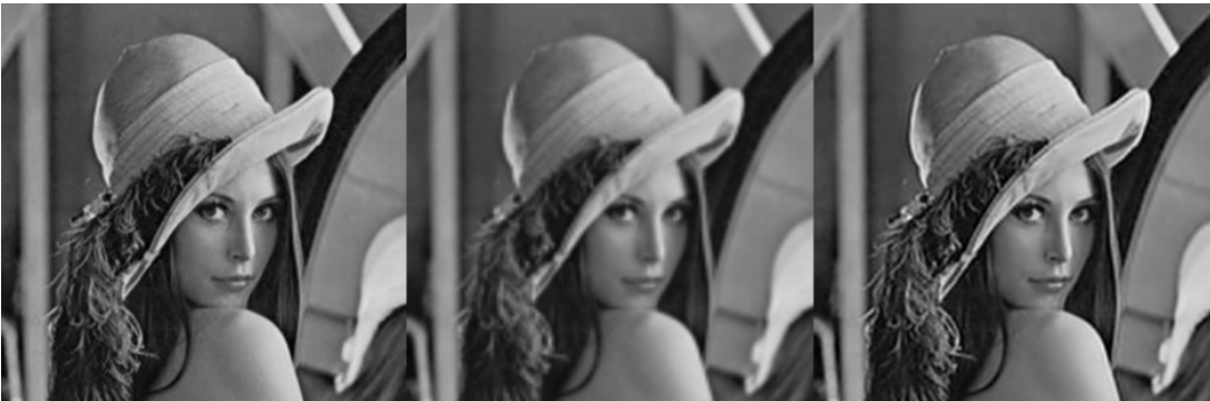
Fig. 2.4 Comparison between interpolation and POCS (left: Original Image, Middle: Bilinear interpolation, Right: POCS algorithm)
