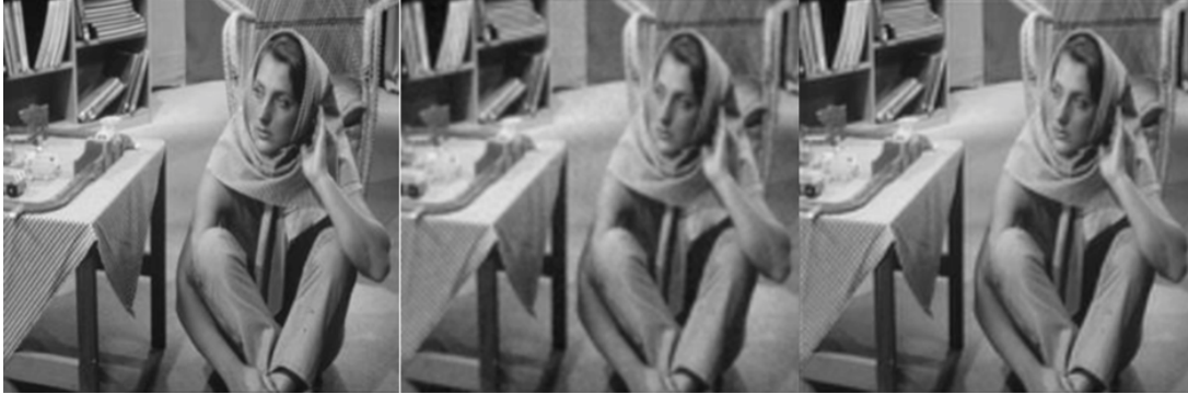
Fig. 2.5 Comparison between interpolation and MAP (left: Original Image, Middle: Bilinear interpolation, Right: MAP algorithm)
