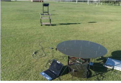
Fig. 11. The circular array used in the experiment and the EMI desktop interference.
