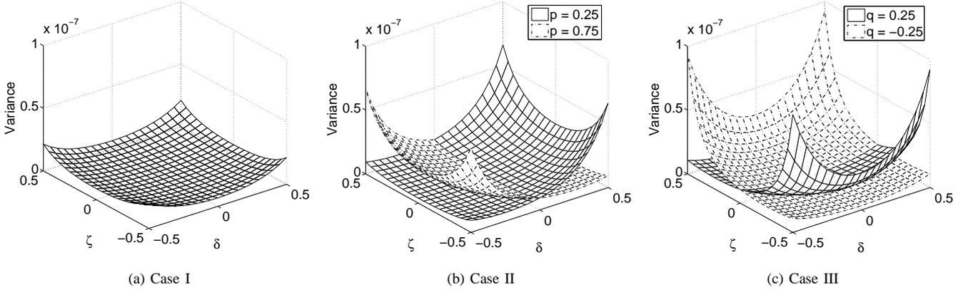
Fig. 1: Theoretical variance of  $\hat{\mu}$  under different values of  $p$  and  $q$  when  $r = s = 1$  ( $\eta = \gamma = 0.01, M = N = 32, \rho = 10\text{dB}$ ): (a)  $p = 0.5, q = 0$ ; (b)  $p = 0.5 \pm 0.25, q = 0$ ; (c)  $p = 0.5, q = \pm 0.25$ .
