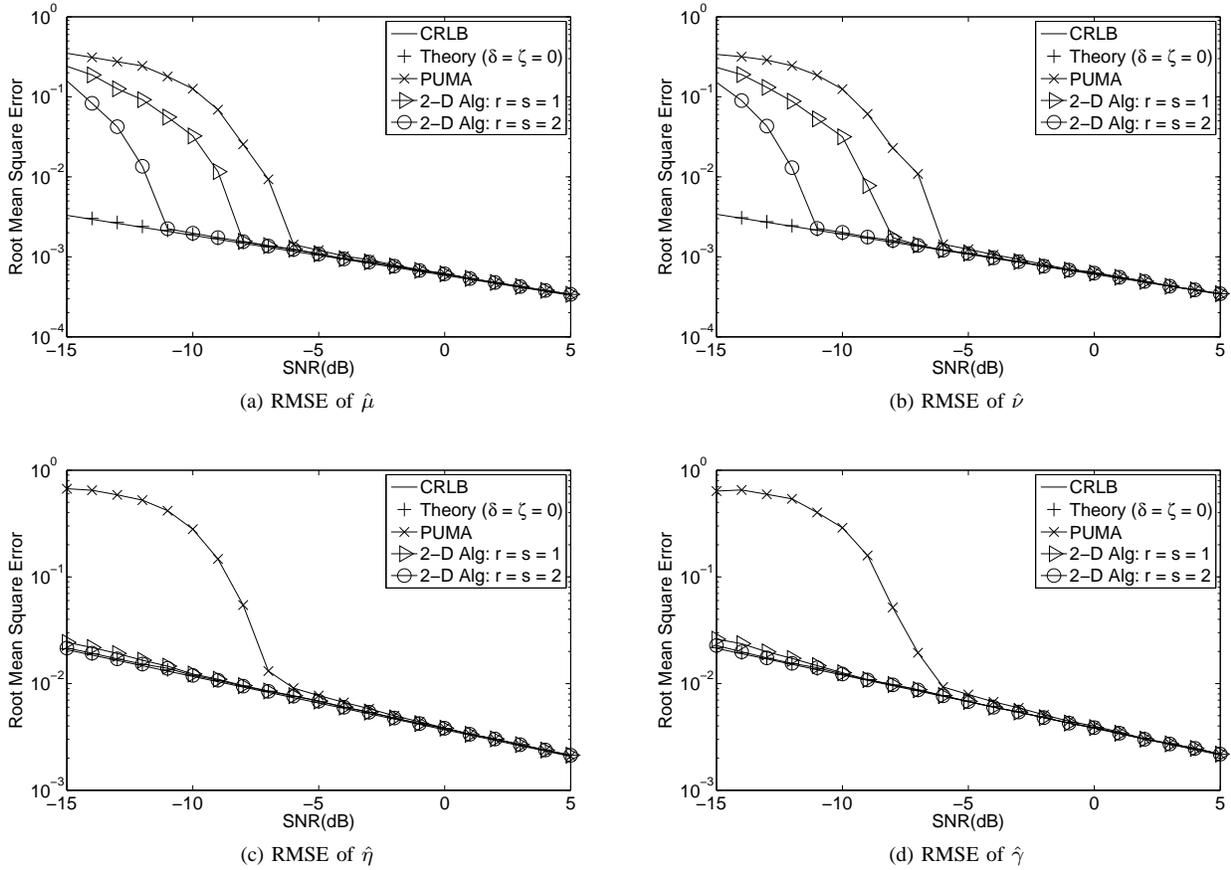
Fig. 2: RMSE of different estimators versus SNR when  $\eta = 0.01$ ,  $\gamma = 0.02$  and  $M = N = 32$ .
