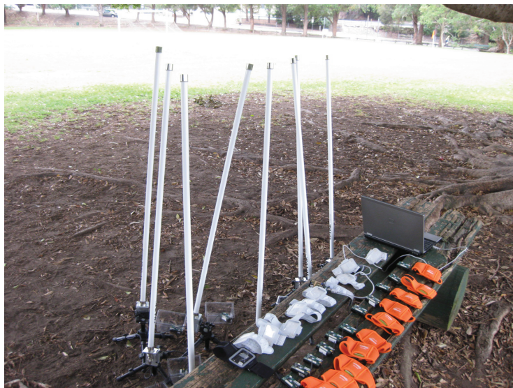
Figure 1: Equipment used in the experiments: Motes and GPS units for each player, and 8 base-stations with high-gain antennas
