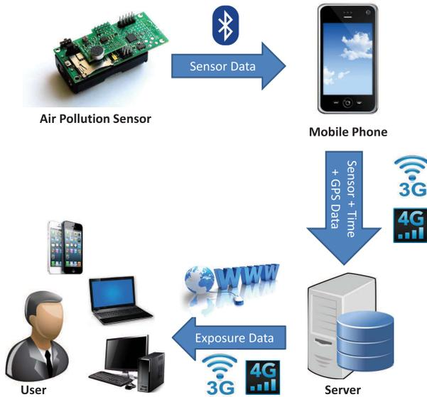
Fig. 1. HazeWatch System Architecture.
