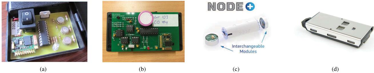
Fig. 2. Air pollution sensor: (a) Metal Oxide sensor; (b) Electrochemical Sensor; (c) Node Sensor; and (d) SensorDrone Sensor.
