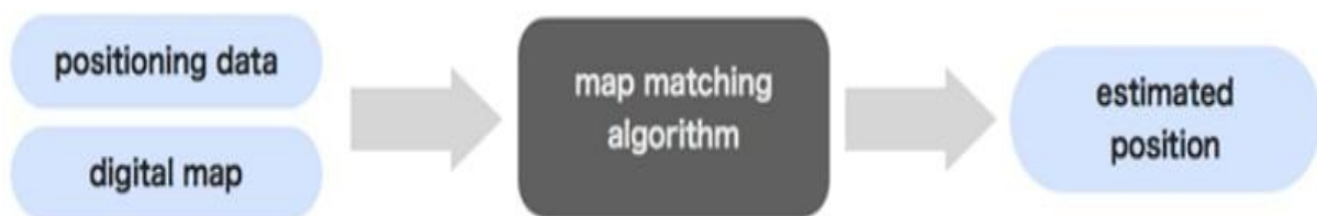
Figure.11 Block diagram of map matching process [13]
