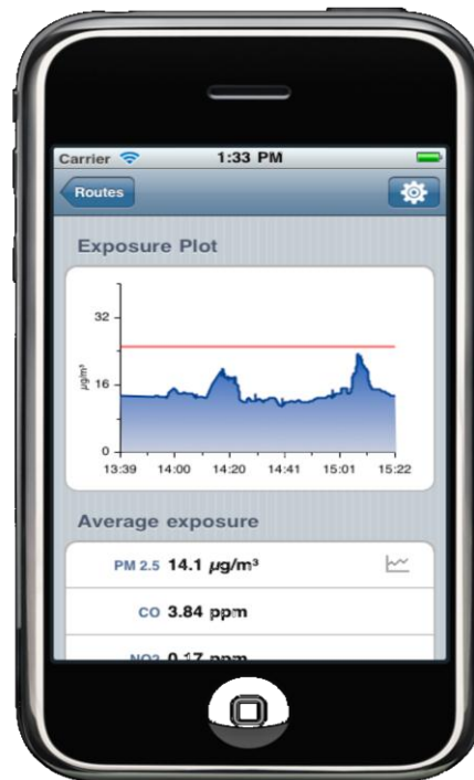
Figure 8: Screenshot of personal pollution exposure application running on an iPhone. Pictured is a graph of PM 2.5, with the guideline value (WHO) plotted in line[8]
