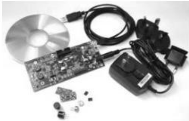
Figure 37: E2V metal oxide semiconductor gas sensor evaluation kits
