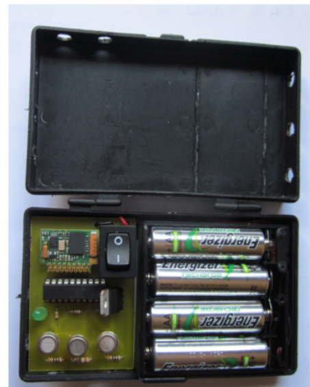
Figure 2.7 Wireless sensor board
