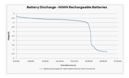
Figure 11: Battery Discharge curve
