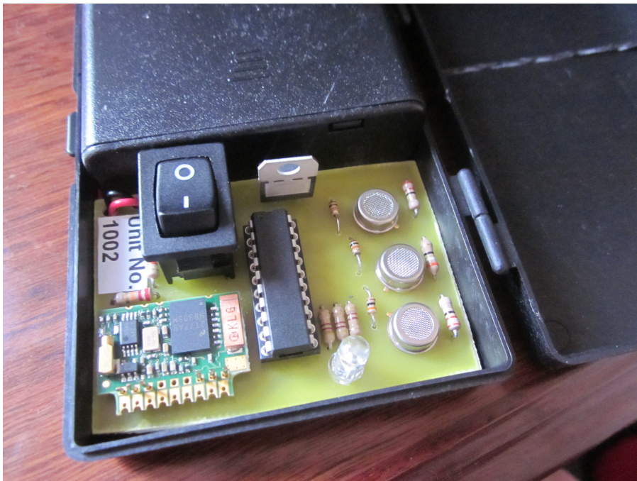
Figure 13: Mobile pollution sensor hardware
