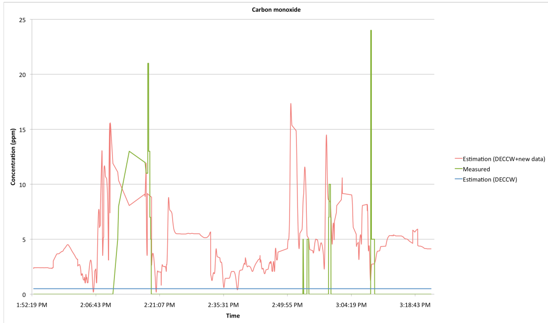
Figure 38: Graph of carbon monoxide concentration as i) estimated using DECCW+experimental data, ii) measured by the GasAlert Micro, iii) Estimated by the DECCW data alone
