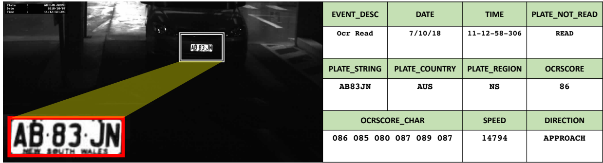
Fig. 1. LPR camera outputs for author's car entering into the campus car park.
